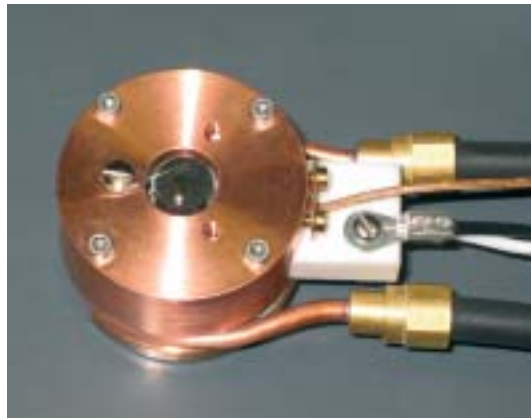
Fig. 2: Heating Stage by Ernst F. Fullam Inc. Centre is the heating element; black tubing is for water-cooling of the heat sink. The heating stage is fitted with a standard dovetail to fit Carl Zeiss SMT SEM stages.
