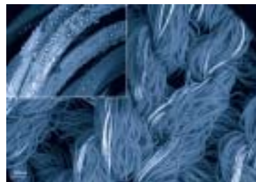
Fig. 12: BSE imaging of corroded polymer fibres in VP mode (12 keV/ 43 Pa chamber pressure). Inset image showing 15x higher magnification.
