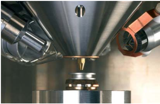
Fig. 2: Photograph of the sharp 80° final lens used on the EVO® MA and LS SEM. The EDS detector is shown at a take off angle of 35° and a working distance of only 8.5 mm. The Everhart-Thornley SE detector is visible behind the EDS detector.
