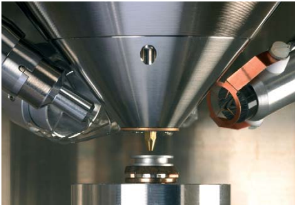
Fig. 6: Inside view of the EVO® chamber, showing the BeamSleeve® in place on the objective lens.
