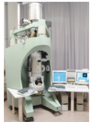
Carl Zeiss SMT's sub-Ångstrom ultrahigh resolution transmission electron microscope with revolutionary column suspension concept.
