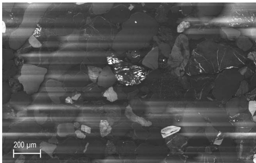
Fig. 2: Polished section including carbonates imaged with a standard CL detector. This streaking effect is associated with persistent luminescence from carbonates. 15 kV
