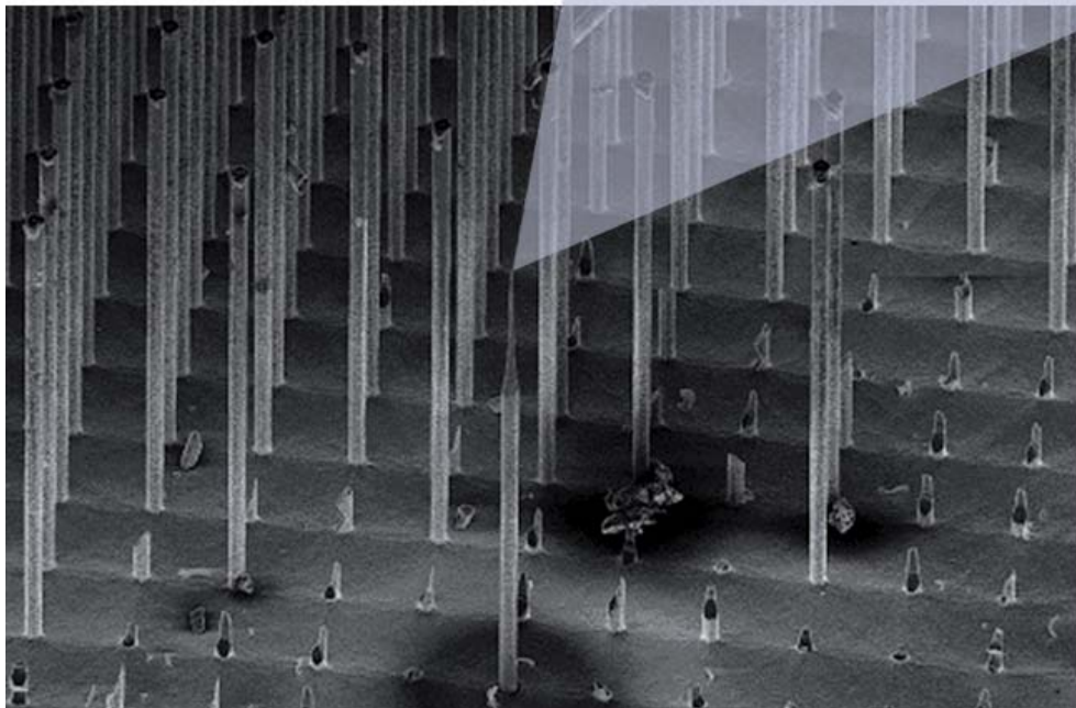
Figure 3: Overview of large aspect ratio Si Posts fabricated by Reactive Ion Etching. The Si post in the front was trimmed by Annular Milling (Sample courtesy of E. Cadel, University of Rouen, France).
