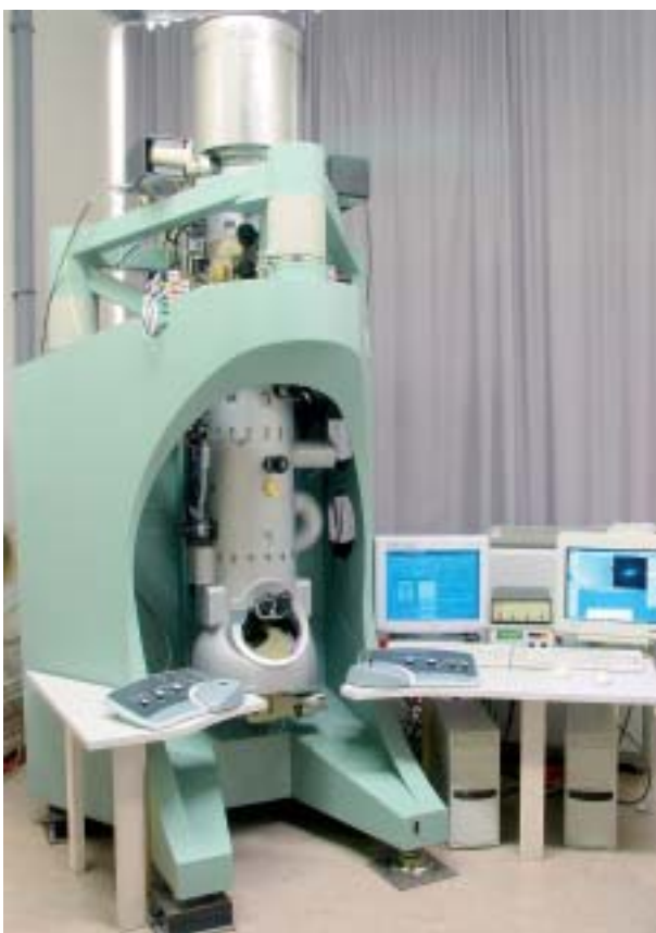
Fig. 2: Carl Zeiss SMT's newly developed sub-Angstrom UHRTEM with revolutionary column suspension concept.
