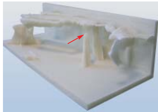
Fig. 1b: From nanometers to centimetres: Stereolithographic reconstruction of the recorded 3-D data in PMMA. The size of the solid plastic model is about 0.3\text{m} \times 0.1\text{m} \times 0.1\text{m} . Note the excellent resolution on the small interconnect (arrow)
