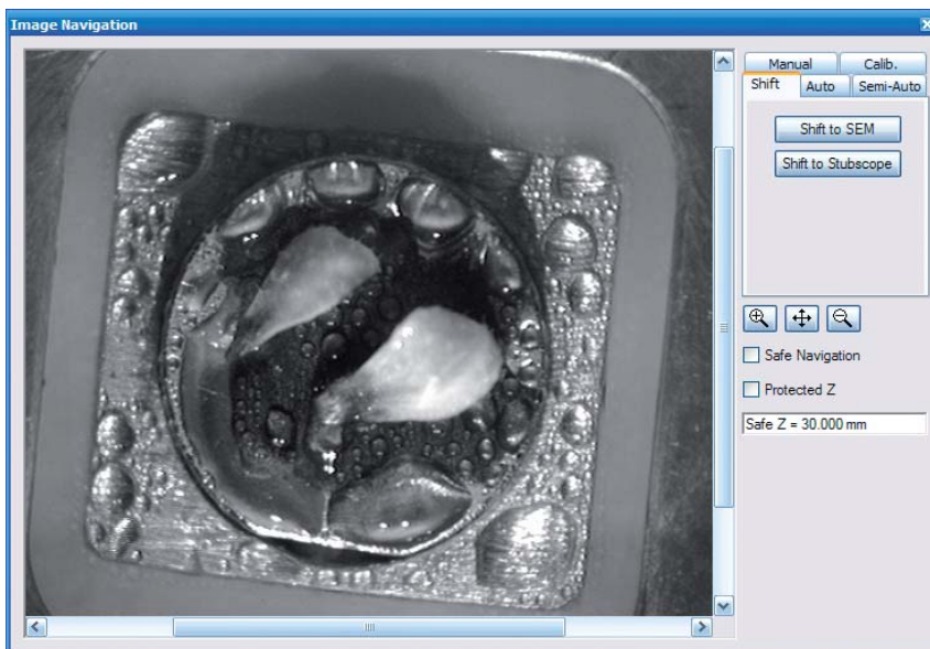
Fig. 6: Seeds on Coolstage with water drops confirming humid conditions are achieved
