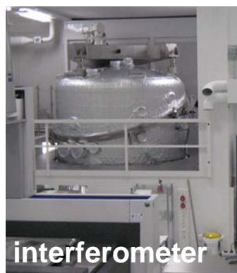
Figure 11 System wavefront interferometer at EUV wavelength. The vacuum vessel can be opened completely to allow to insert six mirror scanner optical systems. On the right hand side, the reproducibility of the wavefront measurements is shown.
