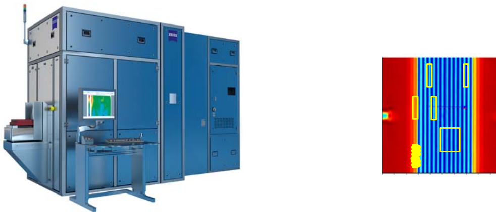
Fig. 2: The newly developed WLCD tool for in-die mask CD metrology using aerial imaging. Multiple ROIs can be placed in the field of view to measure the CD on arbitrary features
