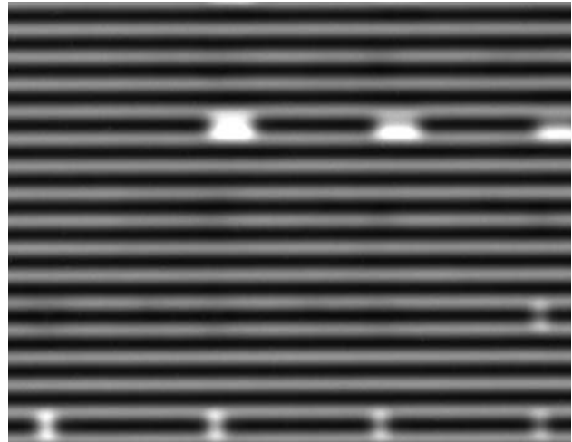
b) Aerial image after the repair of nine defects
